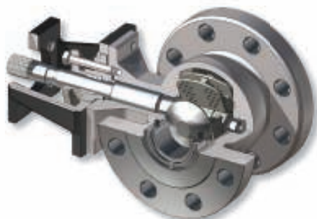
FIGURE 5. The simpler internal structure of rotary valves when compared to linear valves makes them more suitable for service where impurities are present in the fluid
