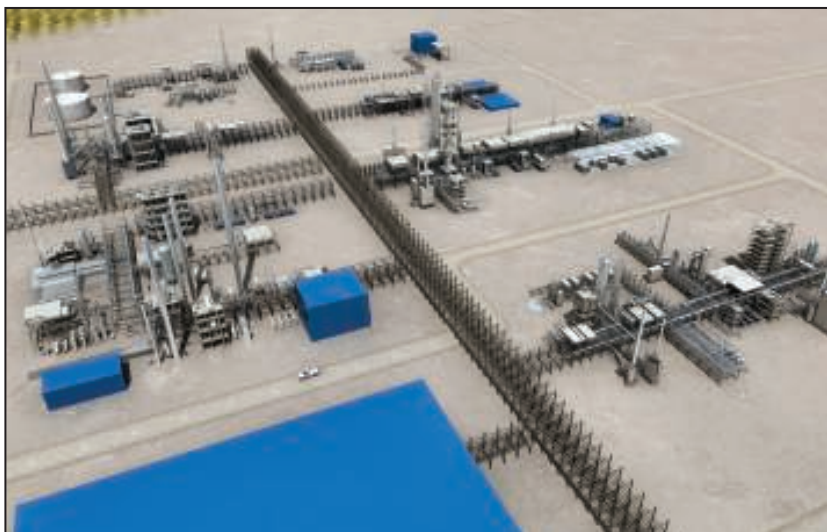
FIGURE 3. Engineering teams should consider using software to generate images in 3D format, since this can help the team to visualize the complete plant layout from laydown areas and roads to the equipment, structures, piping, electrical locations and so on
