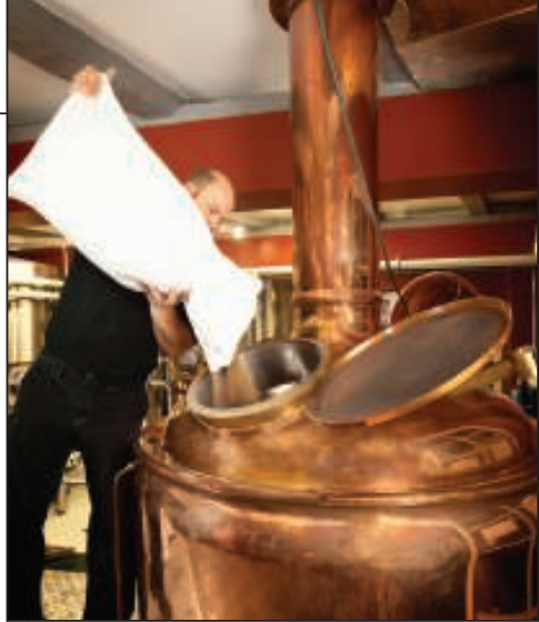
FIGURE 3. Extra care must be taken any time personnel have direct contact with potentially combustible dusts or solids, for example, when pouring a bag of reactant into a vessel
