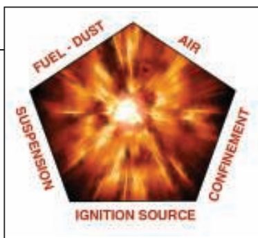
FIGURE 4. The dust explosion pentagon represents the conditions that can lead to a catastrophic event
